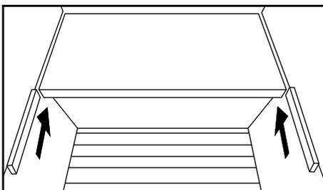
**Optional:** After the bench is installed, you can slide in the included wood pieces to prevent the bench from sliding left to right. One piece can be placed on each side next to the bench. If you decide to flip the reversible bench over, please remove the wood pieces first.
